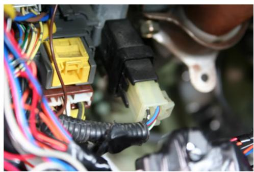
**Step 4:** Disconnect the plug, and Connect the other end of wire that is connected to your pen clip or brass fitting, or whatever piece of metal you used to make contact to the back of the hub, to the power connection in the plug which looks like this:
