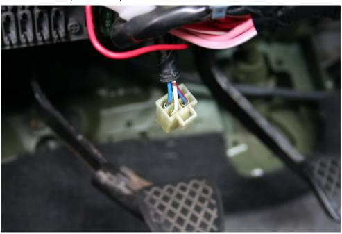
I stripped it out, and shoved it in the female connection of the plug, you should be shoving it in the blue/red connection of the plug above. That is what gives power for the Horn.
