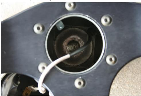
**Step 6:** Re-install your steering wheel, by tightening down the 19mm nut and make sure it lines up good with how the <u>tires</u> are facing, if not take it off and line it up correctly. Also install all plastic garnish pieces and you should be set!
