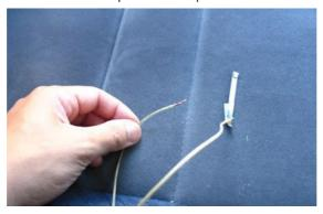
You have to find a way to secure it so it makes constant contact to the backing of the hub, as thats where the plug inside your hub gets its power from.
