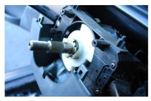
**Step 2:** What you will need to do following taking off the steering wheel, is connect a wire to a piece of metal like a pen clip or the brass piece which 88-91 Civics( Part # PART #35259-SH3-A02 For those interested) used, to get contact and power to the horn. Mine Looked similar to this:
